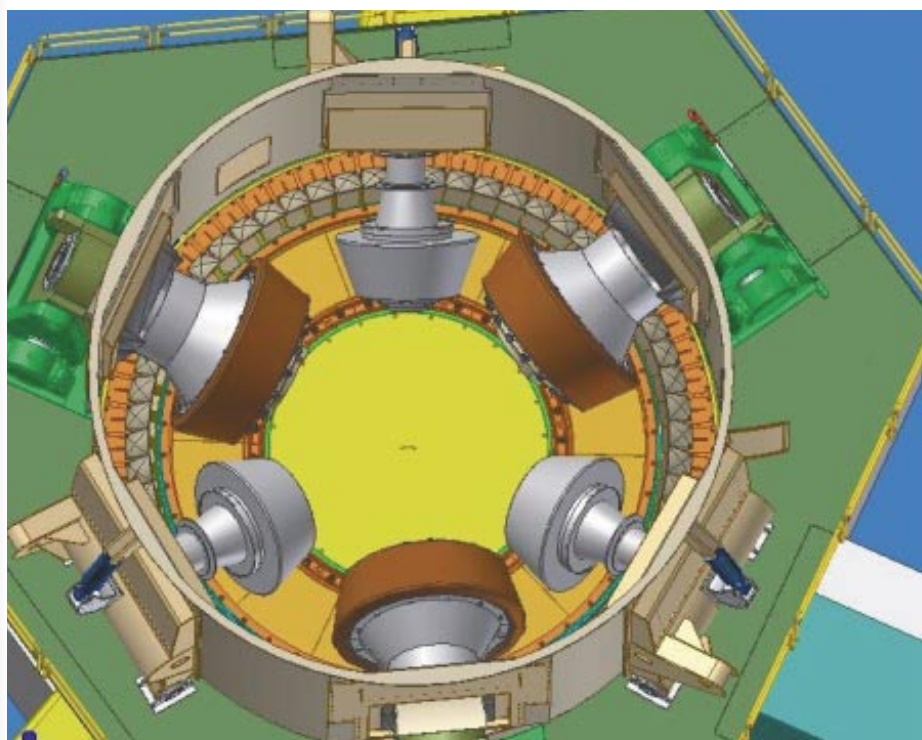
Figure 2: Arrangement of the three master and three slave rollers in the LM 56.3+3 CS mill.
