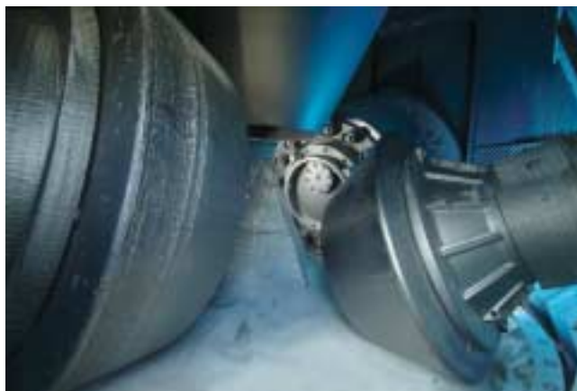
10 2+2 Technologie – Die Support-Walzen bereiten das Mahlbett vor, die Master-Walzen mahlen das Material 10 The 2+2 technology – The support rollers prepare the grinding stock while the master rollers do the grinding
