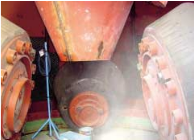
8 Walzen neu 8 Rollers with new grinding parts
